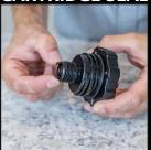
Squeeze tabs and pull retainer out.
