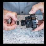
Reinstall retainer and seal.
