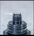
Make sure retaining tabs are fully pushed out and seated properly.
