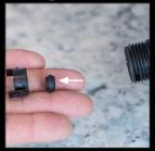
Inspect cartridge seal for cracks or defects. Replace if needed. Note orientation when removing.
