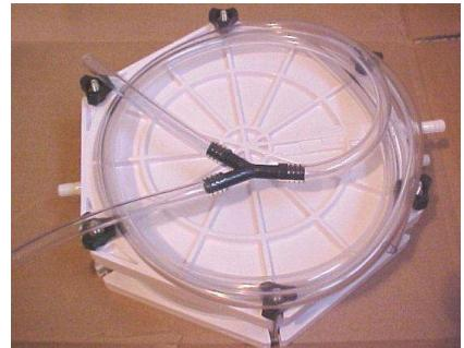
Allow the filtering plates to soak in water for a few minutes. Make sure the intermediate ring is nicely in the middle. The nuts and bolts are then fitted and tightened. Remember that the nuts must all be equally tightened, so we alternatively tighten two on each side. Connect the outlet of the container to the filter inlet (separator) using a PVC hose. Fill the container with water to a maximum of the 11.4 litre mark, screw the pump on it and start pumping.
